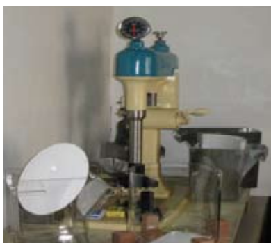
Metso D12 Laboratory Flotation Machine will do multi tasking, lab size, agitator and scrubber.
