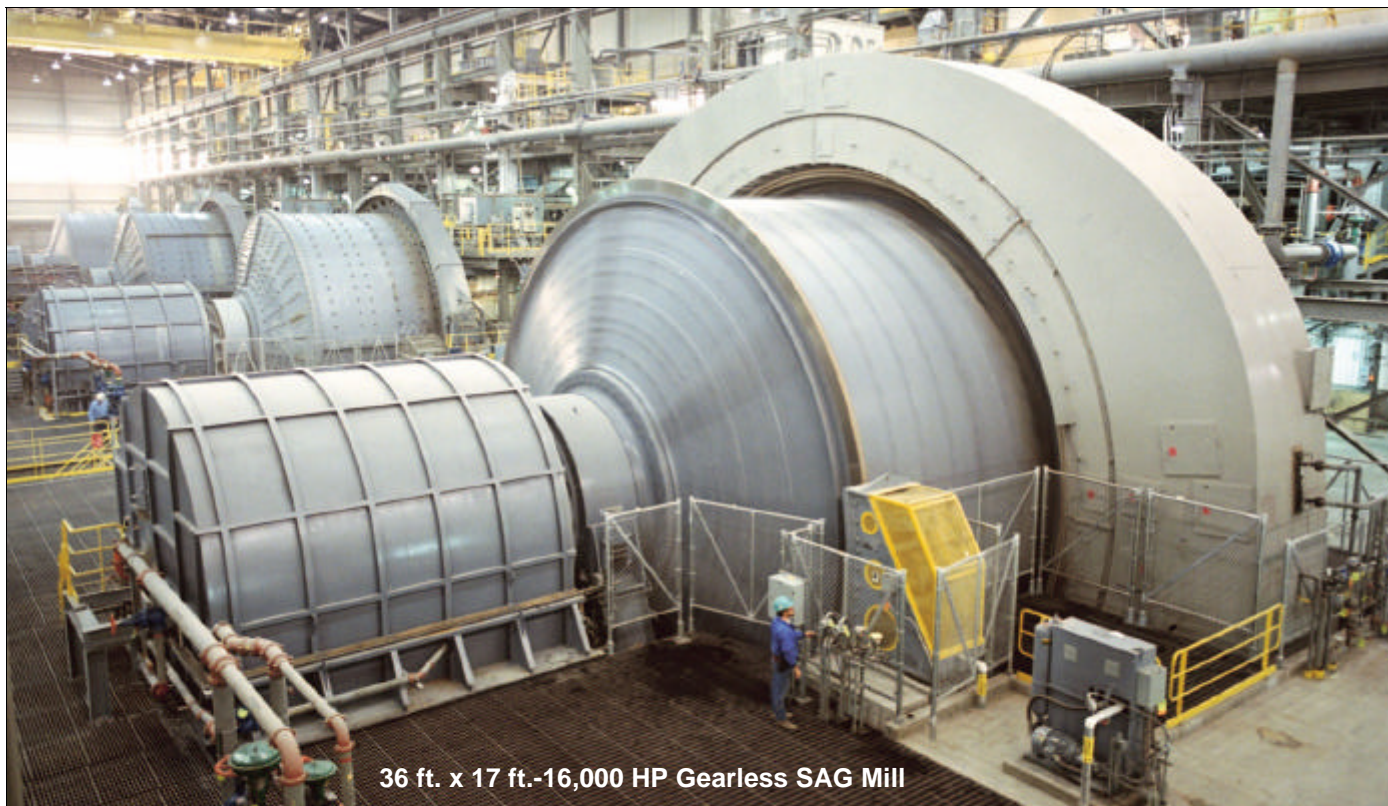
36 ft. x 17 ft.-16,000 HP Gearless SAG Mill
