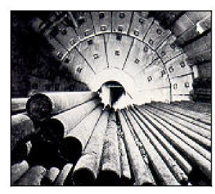
entrance of the feed to the grinding charge uniformly. This permits maximum grinding efficiency at the maximum rate possible before an overload occurs. In addition, this type of head construction permits the use of rods the full mill shell length, and reduces wear on the end liners.
