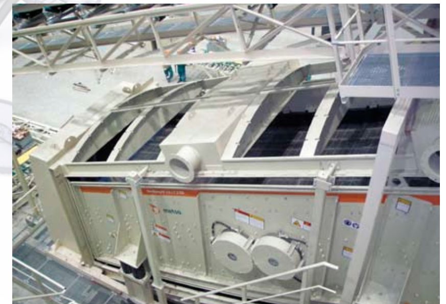
Screen matched with Trellex media and dust enclosure
