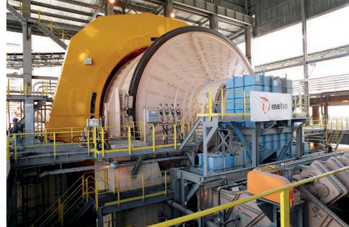
SAG mill matched with 3.6 m x 7.3 m DD "super screen"
